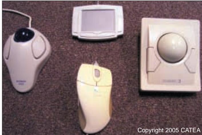
*A variety of mouse alternatives are available, including trackballs (left and right), a track pad (top), and a contoured mouse (bottom).*
